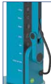
Buttons for: LED light, color filter, image rotate, zoom, exposure, auto-focus, power
